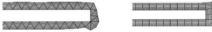
Fig. 5. The two closed surfaces surrounding the inner armature of the transmission line are shown for the two mesh topologies.
